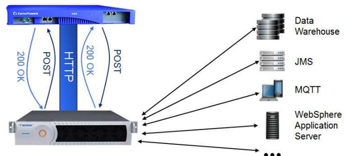
To enable high message rate between DataPower and Solace, multiple parallel HTTP connections are used in both directions. This avoids the round trip performance limitation of blocking HTTP requests, which unlocks the full capacity of the Solace message router. The use of bidirectional HTTP POST requests removes the possibility of message loss which can exist when using HTTP GET requests to poll for messages.
