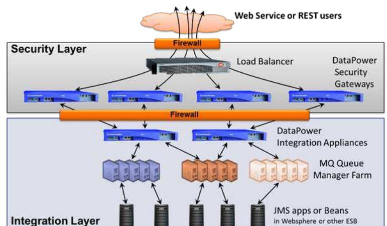
Such systems usually experience volatile and unpredictable peak demand, so companies need to load balance incoming traffic, and horizontally scale the security and integration layer across many appliances to accommodate peak volumes and provide fault tolerance.
